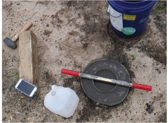
Figure 4.4.1-1. 6-inch and 12-inch Double Ring Infiltrometer
